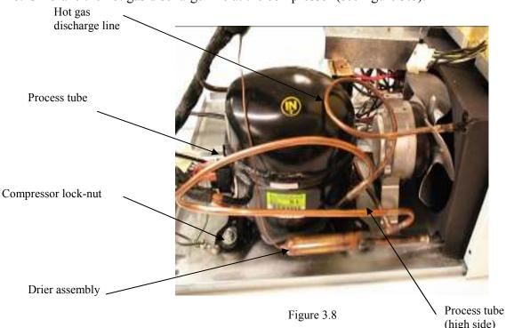
26. Un-braze the hot gas discharge line at the compressor (see figure 3.8).
