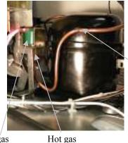
Brazed joint (evaporator bypass tube)
